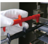
For clamping around the target busbar
