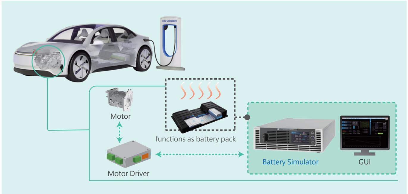
Start-stop system motor driver test application
