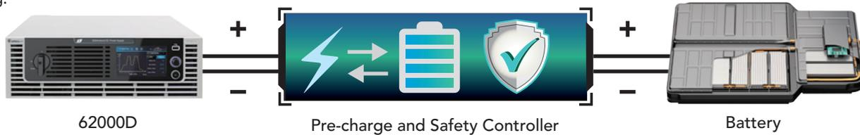
\* When using the 62000D to connect the battery, it is necessary to add a safety pre-charging circuit to avoid inrush current once the battery is connected, and protect the battery and equipment. For battery charge-discharge mode, please contact Chroma office.
