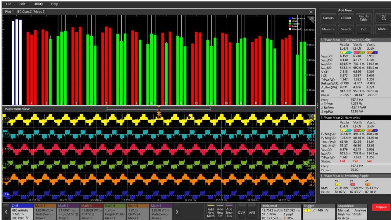
The harmonic plot indicates passing harmonics test results. Each set of bars contains results for phases A, B, and C for easy correlation. The set of green bars indicate a pass and the red bars indicate a fail.
