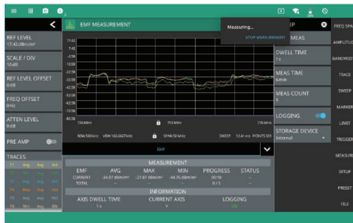
EMF Results Show Power from each Antenna Axis and Summary Results for Peak and Average Power over a Defined Time Period
