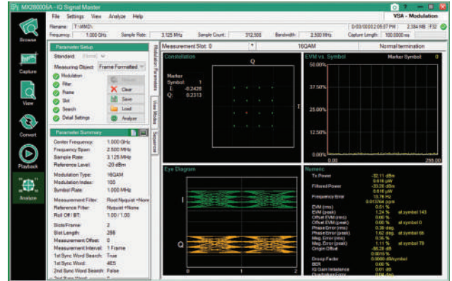
MX280005A Single Screen Multiple Results Vector Signal Modulation Windows
