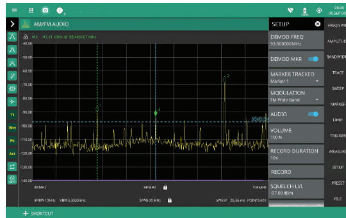
AM/FM Signal Demodulation at Marker Frequency
