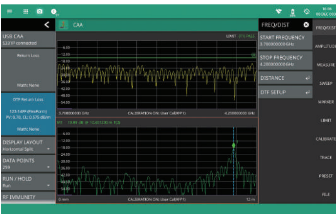
Simultaneous Display of Cable and Antenna Return Loss and Distance-to-Fault (DTF)
