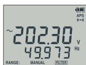
With low-pass filter on
