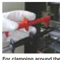
For clamping around the target busbar
