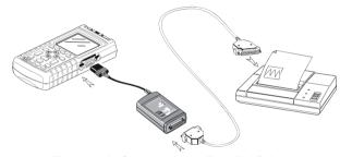
Figure 7-2. Connecting a Parallel Printer
