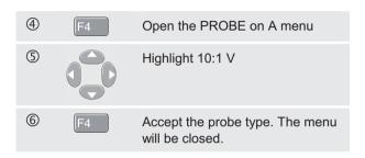
Observe that the 10 times attenuation of the Probe is compensated in the voltage readout.
