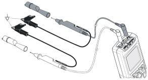
Figure 9-2. Grounding with Short Ground Lead
