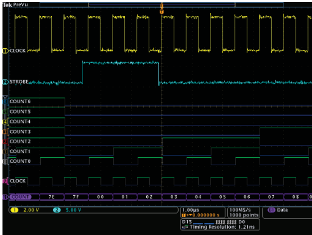
The MDO4000C Series provides 16 integrated digital channels enabling you to view and analyze time-correlated analog and digital signals.
